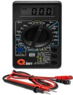
**Multimetro Digital Qian QAD-90011 QIAN MULTIMETRO DIGITAL PANTALLA LCD DE 3 Y MEDIO DIGITOS MUESTREO 2 VECES X SEGUNDO BATERIA 9V NEDA O 6F22 INCLUIDOS MOD. QAD-90011**
