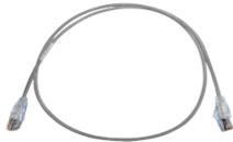
**PATCH CORD UTP CAT6A BELDEN CAD1108003 FORRO PVC GRIS CMR-RISER 4 PARES CALIBRE CONDUCTOR 28 AWG DIÁMETRO REDUCIDO COBRE ESTAÑADO MULTIFILAR USO INTERIOR PARTES RELACIONADAS CONECTORES MODULARES CAT6A PATCH PANEL CAT6A LONGITUD 3 PIES 90 CENTÍMETROS**
